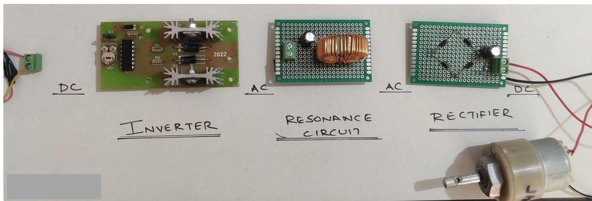
The above diagram is the hardware prototype for the circuit where the motor is used as an application for the system. The system uses Inverter, resonant converter and a rectifier where it changes DC-AC-DC.
