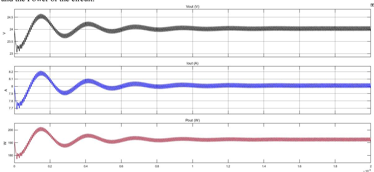
The first graph represented is an Output voltage of 24V, output current of 8A and the total output power of 192W.
