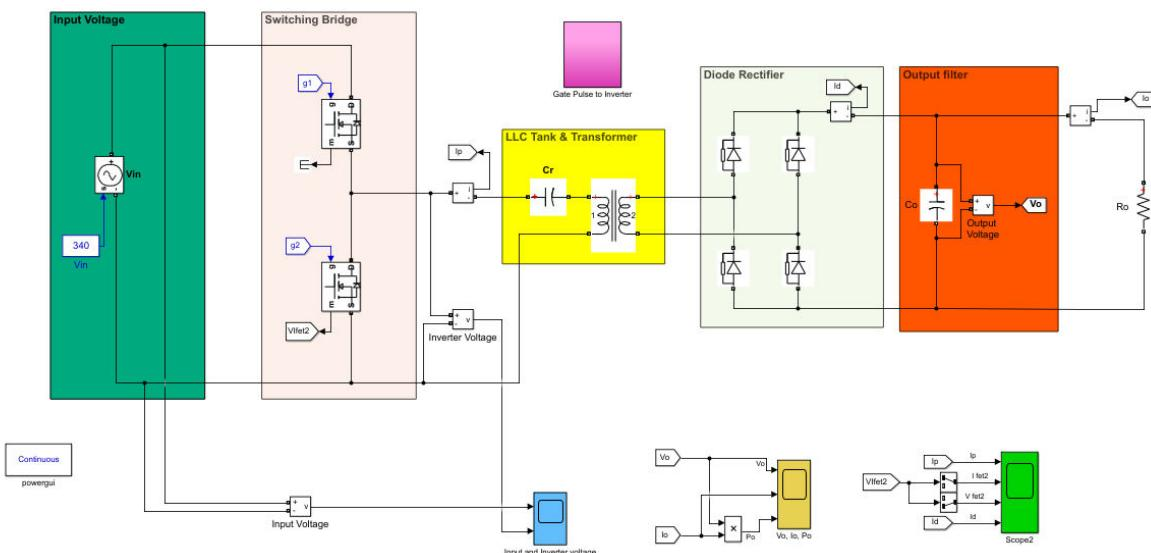
The input to the circuit is of 300V given by DC source. This is given to the inverter which converts DC to AC power. The inverter uses only two switches for the conversion. This becomes a reduced circuit. The pulses are 180° phase shifted. There two gate pulses given to it from the pulse generator of frequency 75 kHz as shown below.
